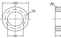
Coating Breakdown Voltage: 1000V, 0.5mA, 2Sec
